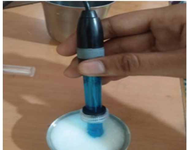
Fig. 5: Testing pH of Milk through pH sensor
